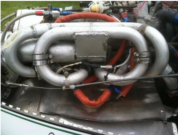
The photo above shows Dennis's very creative intake manifold plumbing. This is a tuned intake to give him max power/efficiency at cruise settings. His engine is a stock 2-rotor out of an RX8 automobile. It is very quiet in comparison to other rotaries due to an innovative exhaust system made possible by the RX8 exhaust configuration.
