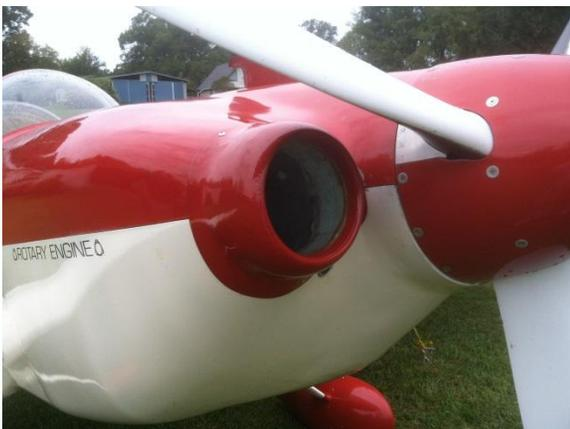
This picture is Tracy Crook's cooling inlet, attention to detail on the shape and contours of the inlet were critical to getting the 260+ HP engine to cool effectively.
