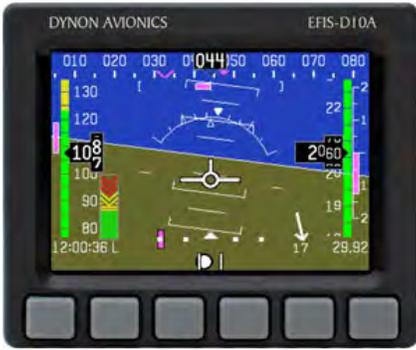
Unique to this STC, EAA worked with the FAA to allow the Dynon EFIS-D10A to be installed without the traditional technical standard order (TSO) or parts manufacturer approval (PMA) requirement.
